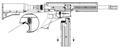
3. REMOVING THE BARREL - (1) Shut off the slide check attached to the tank. (2) Next, remove the magazine from the marker. (3) Slightly push in the barrel and rotate the barrel lock counterclockwise. Then pull down the barrel lock. (4) Your barrel is now free to slide out along the barrel lock track.
