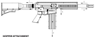
REMOVE HOPPER COVER PLATE - Remove the Hopper Cover Plate by removing the four (4) Cover Plate Screws, (Top two screws H-S 440 3/4, Bottom two screws H-S 440 3/8) by using a 3/32 Allen Wrench.
